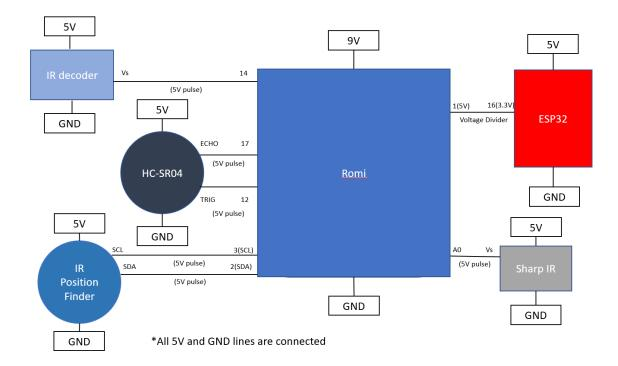
The IR decoder is in port 14, because it requires an interrupt pin so that when we send a signal to it, it will immediately read it via an interrupt. Also plugged into ground and 5V.
